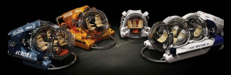
SEAmagine's innovative Aurora technology is a revolutionary approach to submersible design, maximizing the field of view of the spherical cabin and providing an unparalleled vista. The occupants have a view, unobstructed by top hatches and side pontoons, that provide the sensation of entering the underwater world, as opposed to simply observing it.
