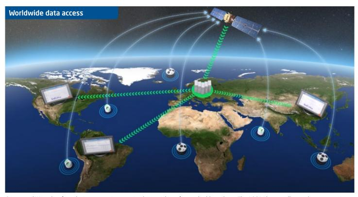
Current and Wave data from the instrument is transmitted via serial interface and cable to shore. The AOS Iridium satellite modem communicates data to the AOS-server, and the AOS-server stores and provides data for presentation on the client website. The data volume and cost is kept to a minimum by focusing on vital data subsets. Full current and wave datasets are stored in the instrument memory.
