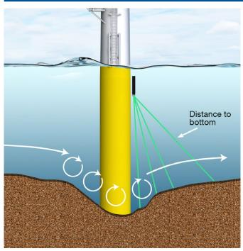
Offshore structures such as wind turbines, rigs, and pilings can be weakened by scour around their base. Scour holes are generated by storms or strong currents and will often appear and disappear on short notice. As a result, storm-driven scour may not leave a detectable signature in a post-storm survey. As such, it can only be properly characterized if monitored also when normal survey operations have to be suspended.
