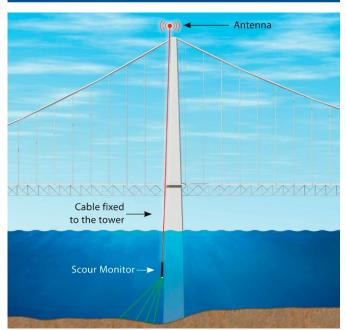
Bridge foundations can easily be undermined by scour, critically affecting the stability and integrity of the structure. An online Nortek Scour monitor, can provide continuous and detailed information about the condition of a pier footings, allowing the appropriate actions to be taken in during storm or flood conditions. It also allows bridge owners to make long term structural studies, for planning and maintenance purposes.
