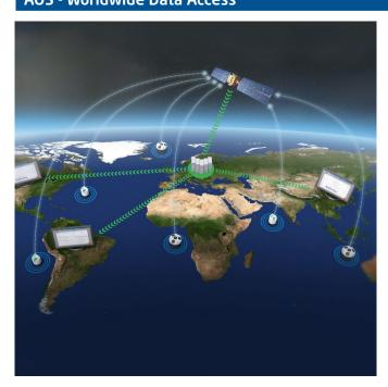
Where there is limited electrical power and communications, the Nortek Autonomous Online System (AOS) makes it possible to power, collect and process data, before transmitting vertical Scour levels via Iridium® to a Nortek server. These real-time Scour levels are ultimately displayed on a dedicated password-protected web site, allowing easy and convenient data access.
