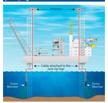
The mobility of the seabed can at times cause jack-up rig operators serious problems. In some circumstances, the legs may become buried or suspended. Both scenarios can be critical. The Nortek Scour Monitor is able to provide an early warning system of such events, allowing time for countermeasures to be taken.
